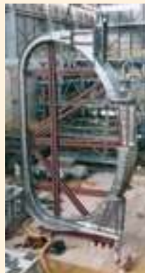
Prototype Vacuum Vessel Sector for ITER – an example of the types of components that will be provided by Europe to the ITER project.
